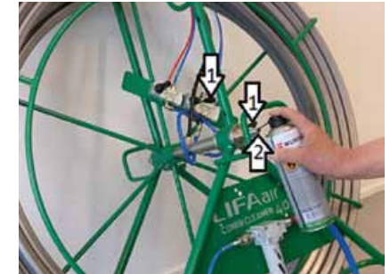
Image 1 1. Open air inlet valve and operation valve. 2. Spray light motor oil* to the air hose connector.
