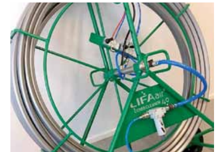
Image 2 Connect compressed air to the connector and run the motor few seconds.
