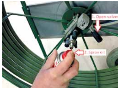
Image 1 Spraying light motor oil* to the air hose connector when the operation valve and air inlet valve are open.
