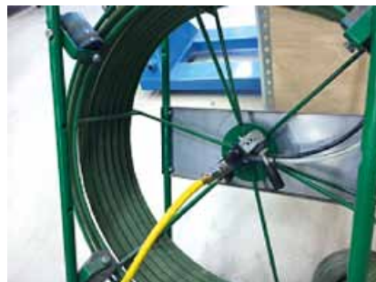
Image 2 Connect compressed air to the connector and run the motor few seconds.
