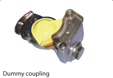
Truck compressed air connection
