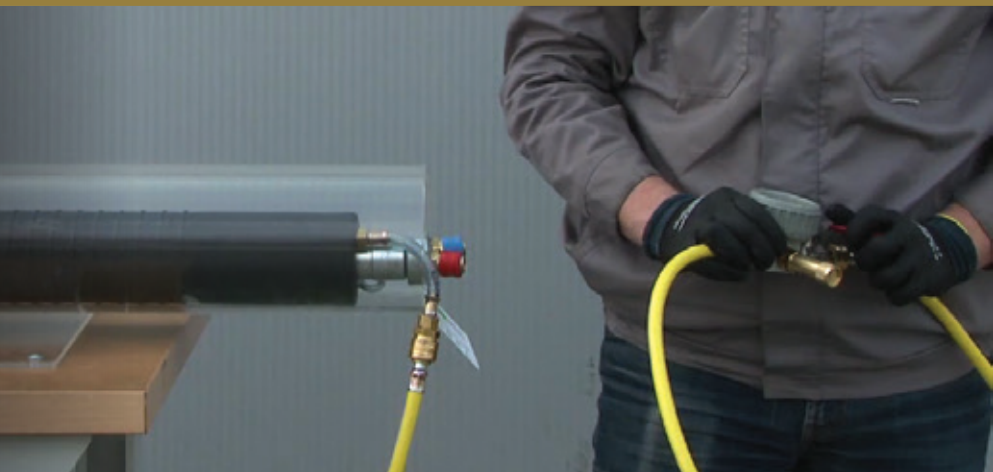
Water test according to EN 1610
