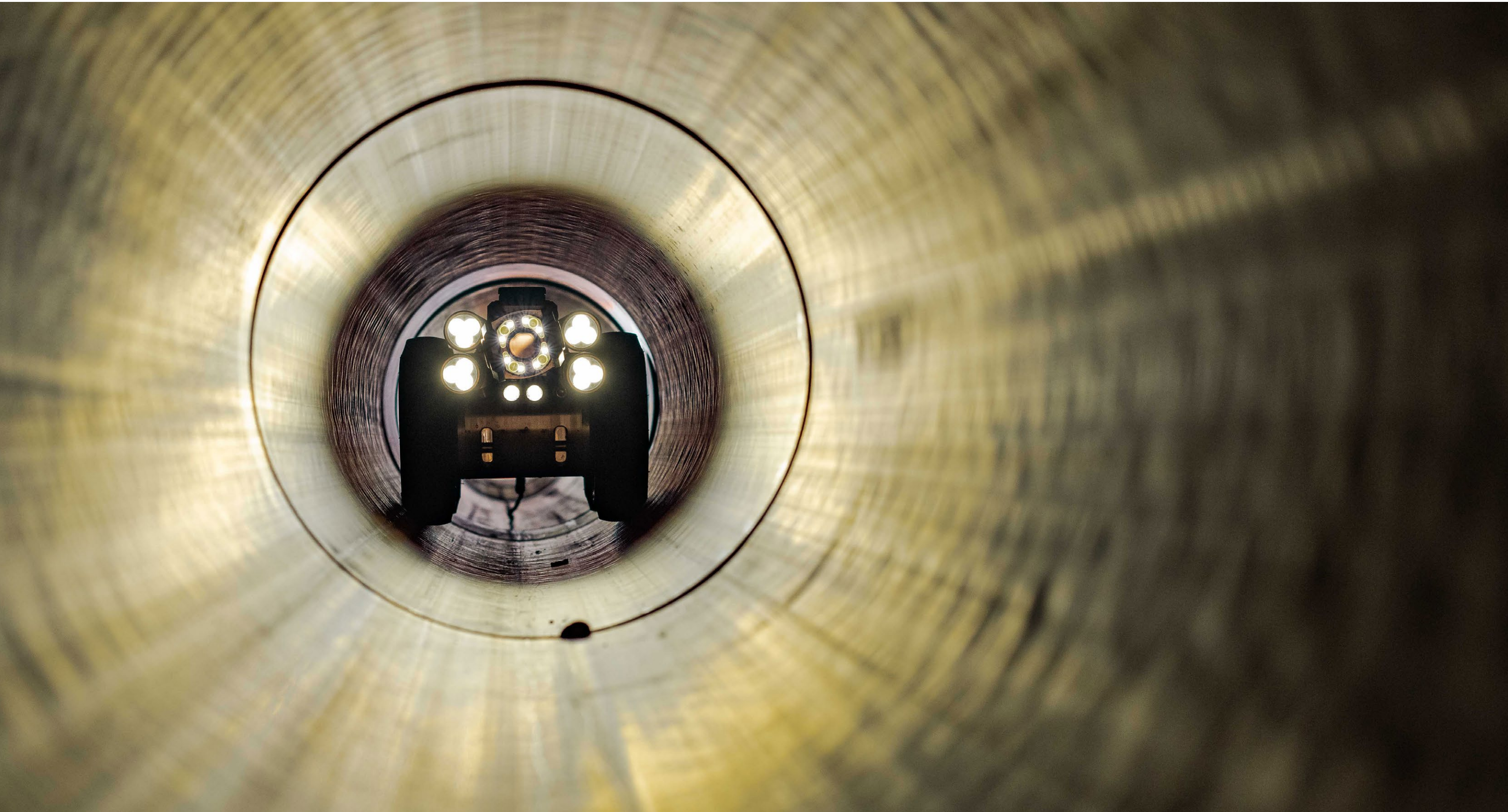
Large diameter RX400 crawler in PVC pipe
