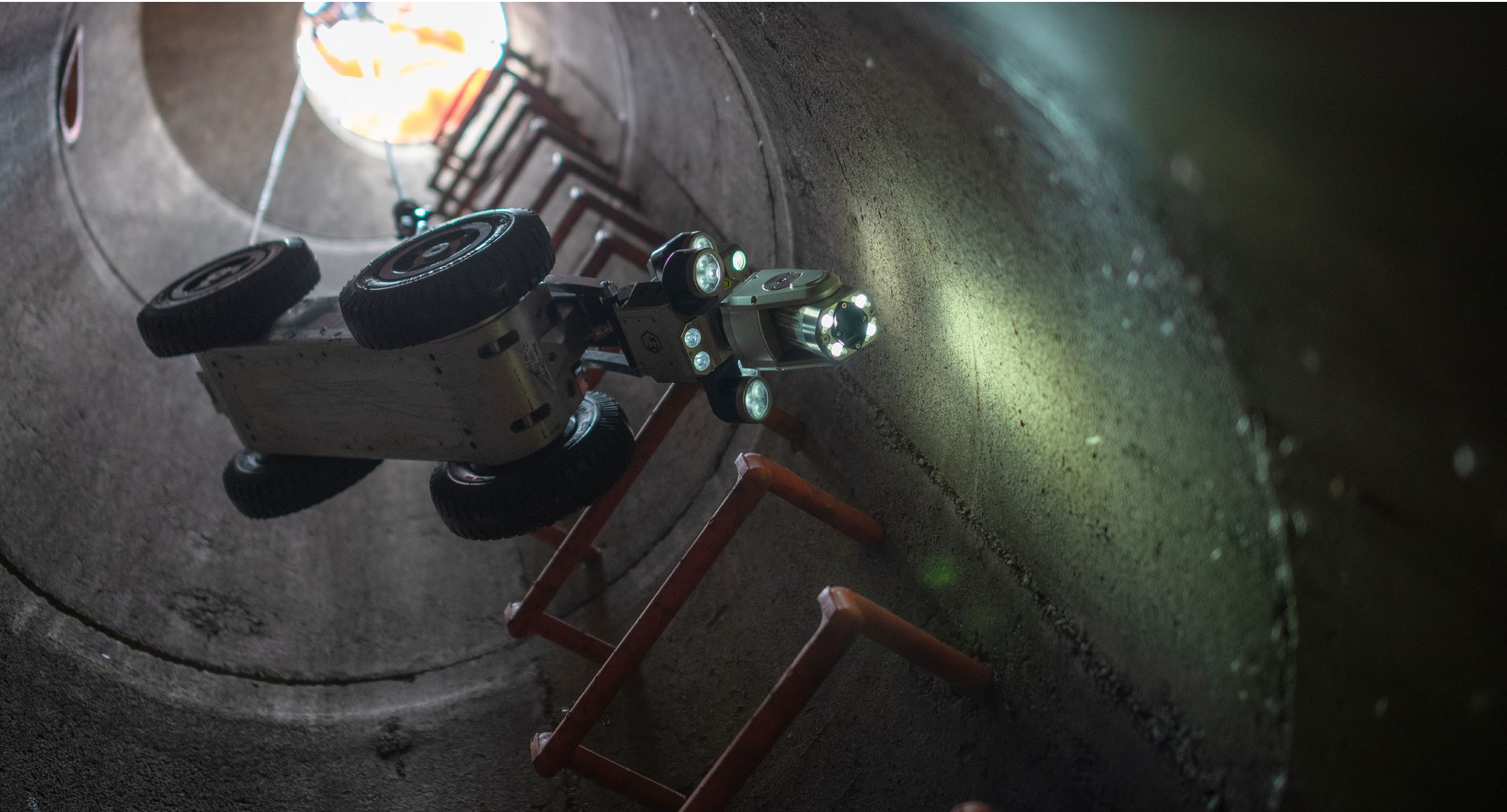
Large diameter RX400 HD deploys in a manhole
